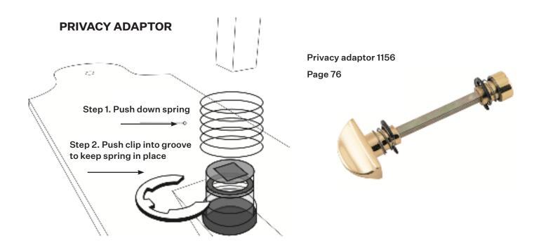
Note: image shows underside of plate
